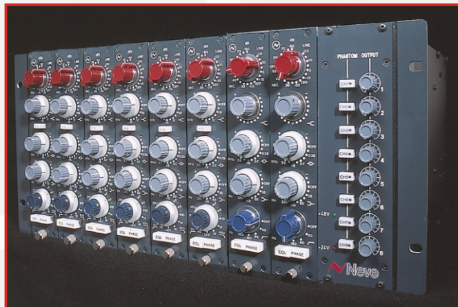
5U rack fitted with two 1073 and six 1084 modules
